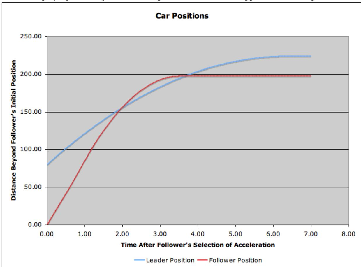
Figure 2: How Realistic Adaptive Cruise Control Can Be Tricky
